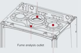
Air intake manifold for split exhaust systems
